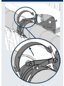
Removing Center Pivot Bolt & Cotter Pin (MacDon, Claas, Honeybee, Geringhoff)
