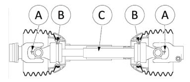
On some 35' and 45' systems (equipped with an extended driveline), there is an additional bearing that requires greasing.
